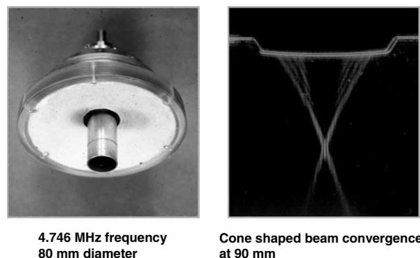
Fig. 2. (a) HIFU transducer. The operating frequency is 4.746 MHz, the diameter is 80 mm and the focal length is 90 mm from the surface of the transducer. (b) Schlieren image of the HIFU beam; the beam converges at 90 mm, the ellipsoidal focal zone is 4.0 mm in length and 0.4 mm in width at the half-power points.
