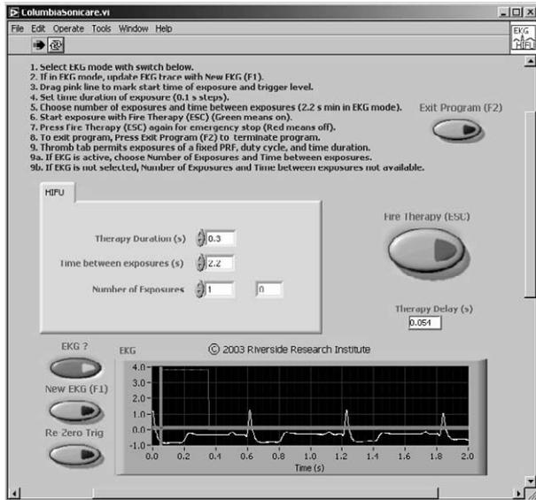
Fig. 3. Main window of the custom software written to control the HIFU system. The pulse duration, PRR and number of pulses can be set with relation to the EKG during in vivo experiments.
