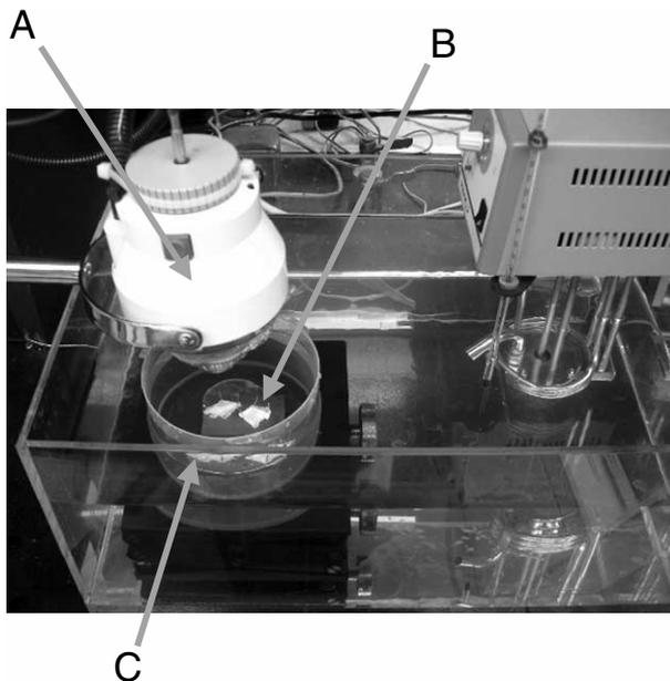
Fig. 1. Experimental setup with HIFU transducer (A). Each specimen (B) was mounted on a rubber sheet and then put in a plastic container (C) filled with degassed PBS. The container was immersed in a water bath with the temperature kept at 37 °C.
